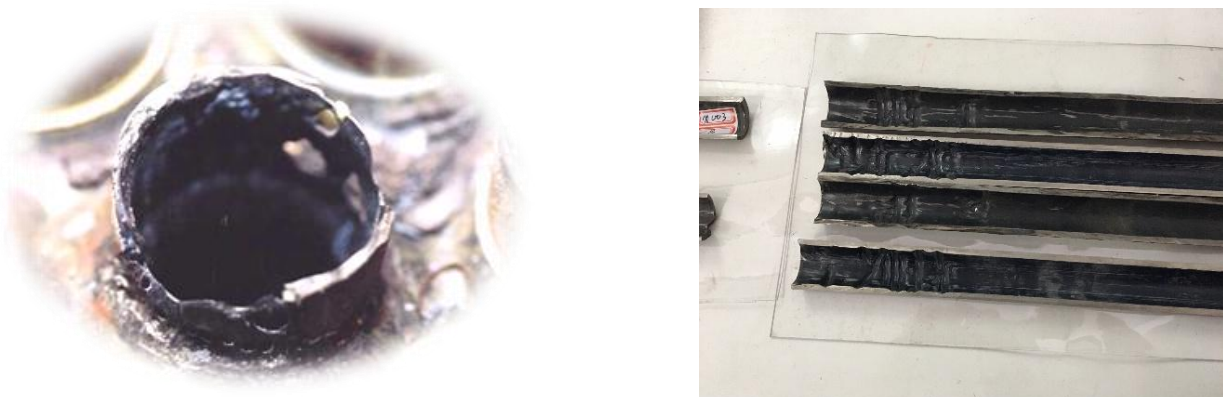
Figure 4: Severe erosion corrosion at the top of a titanium stripper. Left: tube end; right: cross section of titanium tubes.
